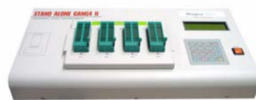
Figure 1-5 StandAlone Gang4 ( for Mass Production )
