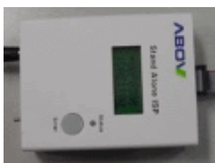
Figure 1-3 StandAlone ISP (VDD power is not supplied)
